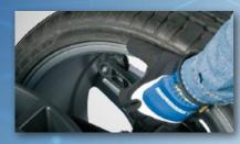
Technicians simply touch the rim with the gauge arm, and the system automatically enters the rim dimensions and selects the appropriate weightbalancing mode.
